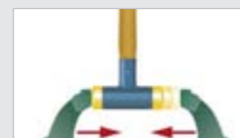
Simple exchange of worn hammer faces: 1. Grip the hammer in the vice, lift to remove old hammer face. 2. Press the new hammer face into the handle until it locks into position.
