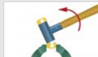
The special metal filling in the hammer casing enables recoilless working.
