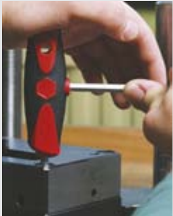
A tool that is a pleasure to use. Using the side blade for even greater torque, a supporting hand stabilises the handle and prevents the blade from slipping.
