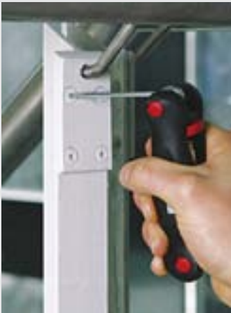
All it takes is three swift actions and you have an effective screwdriver: Pull it out of the pouch, press on the button and set the desired blade to 180° as well as 270°.
